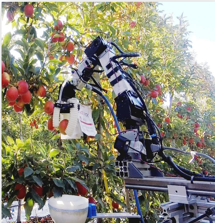
A robotic harvester developed by Dr. Manoj Karkee's team ( https://labs.wsu.edu/karkee-ag-robotics/ ) under evaluation in a commercial apple orchard in Washington State. (Courtesy: Dr. Manoj Karkee)
